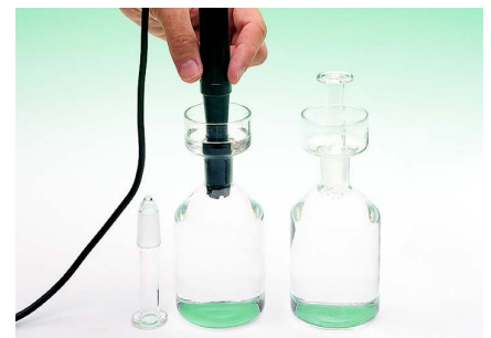
Fig. 2: Karlsruher bottles, preferably used when testing according to the international standard ISO 5815-1 (dilution method). 2)
