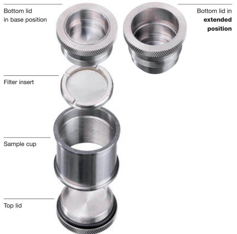
**Fig. 1: Design of the sample cup**
